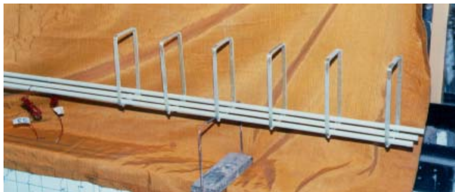
Plate 1 - GFRP reinforcement cage used for tests GB5, GB6, GB9 and GB10
